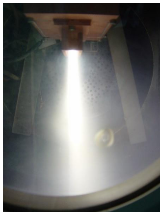
Figure 2. Section view of PBS™ in operation. The confined plasma beam is clearly observed.
